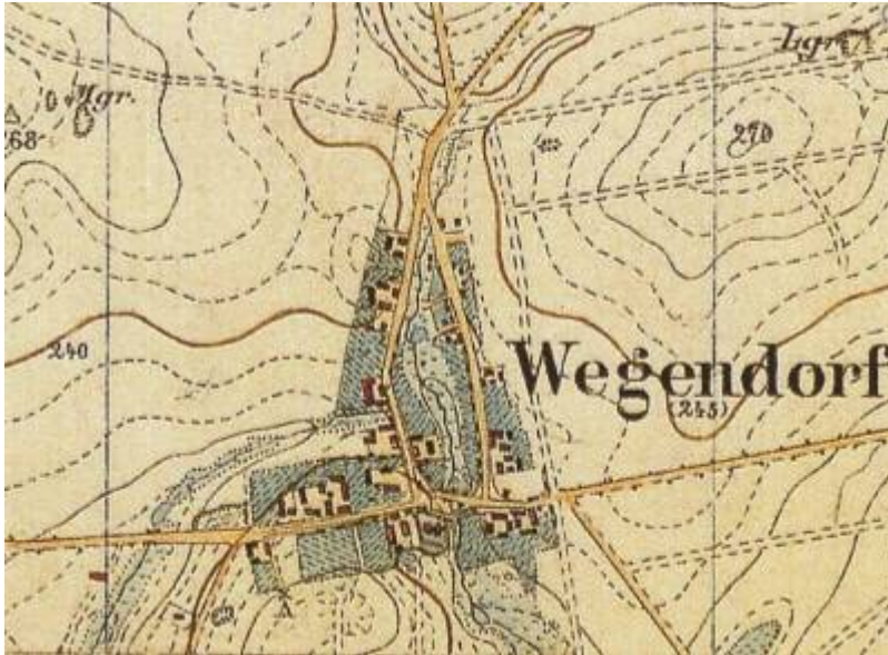
Fig. 13: Indicating elevation contours on a
