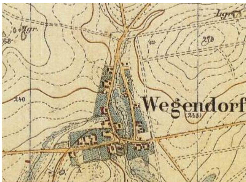
Fig. 13: Indicating elevation contours on a map
