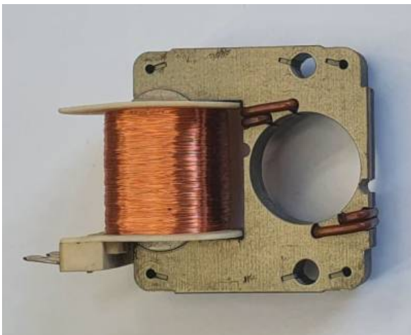
Fig. 25: Core of a shaded Pole Motor
