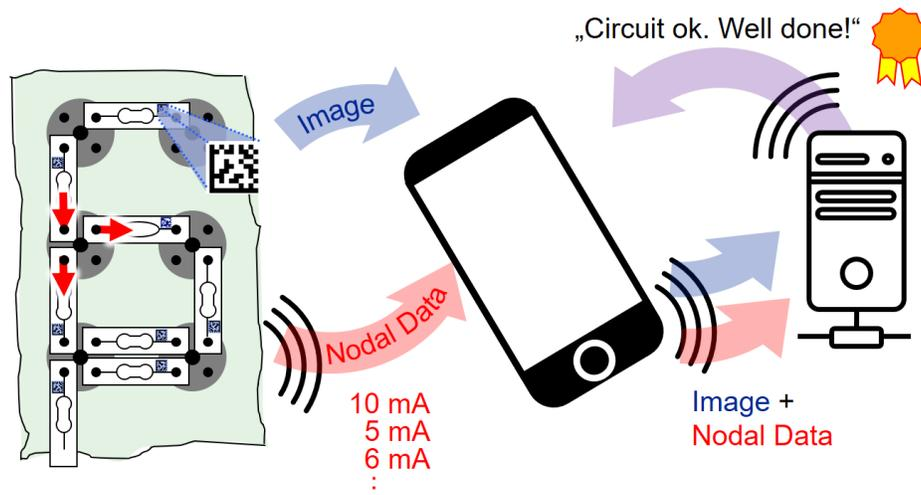
**Fig. 3.** Data transfer of the MEXLEfirst platform: The data acquisition starts on the carrier board (left) on each node (grey full circle). Exemplarily three red currents are shown. These values are sampled and passed through to the server via the mobile phone. Additionally, recorded images are also transmitted to the server. The server analyzes the data and sends a feedback.
