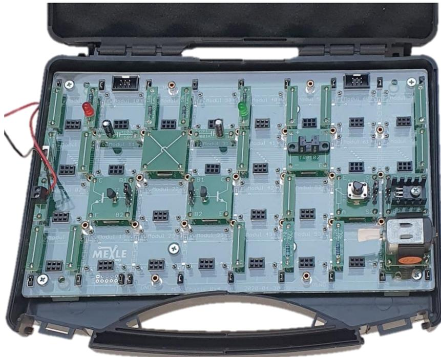
**Fig. 2.** Existing MEXLE carrier board of the lab-in-a-box for the lecture electronics. The circuit on the left shows an astable multivibrator with red and green diodes (on the top). The circuit on the right is a motor driver, which acts on the output from an opto-interrupter. The motor and the power transistor are on the lower right.
